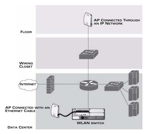
FIGURE 1-1 Connecting APs to the WLAN Switch
