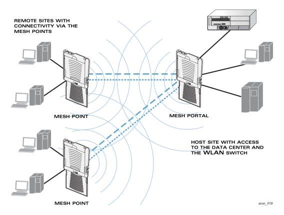
FIGURE 6-18 Sample Point-to-Multipoint Deployment
