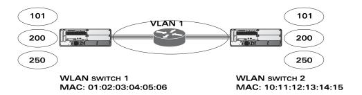
FIGURE 13-37 WLAN Switch-to-WLAN Switch xSec Example
