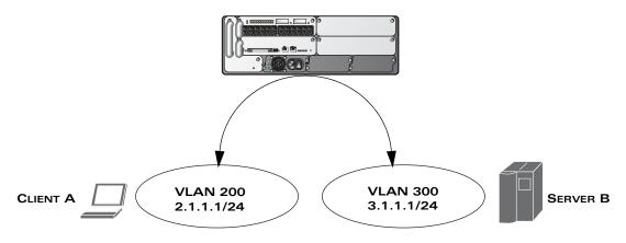
FIGURE 3-9 Default Inter-VLAN Routing
