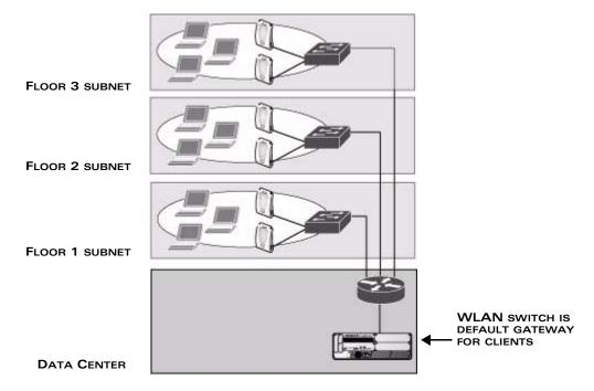
In this deployment scenario, the APs and the WLAN switch are on different subnetworks and the APs are on multiple subnetworks. The WLAN switch acts as a router for the wireless subnetworks (the WLAN switch is the default gateway for the wireless clients). The uplink port on the WLAN switch is connected to a layer-2 switch or router; this port is an access port in VLAN 1.
