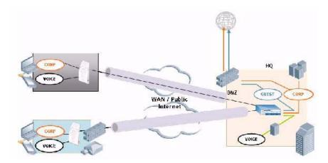
Branch office users want continued operation of the branch office WLAN even if the link to the corporate network goes down. The branch office AP solves these requirements by providing the following capabilities on the branch office WLAN:
