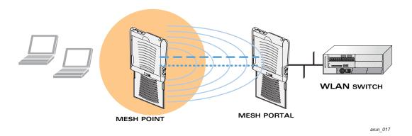
FIGURE 6-16 Sample Wireless Backhaul Deployment
