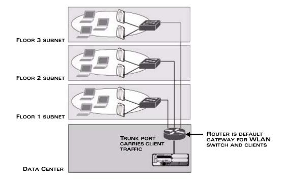
In this deployment scenario, the APs and the WLAN switch are on different subnetworks and the APs are on multiple subnetworks. There are routers between the APs and the WLAN switch. The WLAN switch is connected to a layer-2 switch or router through a trunk port that carries traffic for all wireless client VLANs. An upstream router functions as the default gateway for the wireless users.
