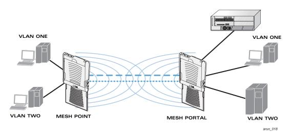
FIGURE 6-17 Sample Point-to-Point Deployment
