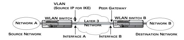
FIGURE 12-34 Site-to-Site VPN Configuration Components
