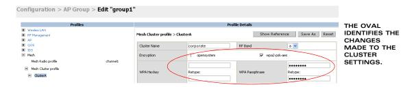
FIGURE 6-21 Configuring the Mesh Cluster Profile Settings
