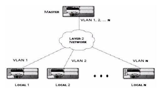
FIGURE 17-45 Redundant Topology: Master-Local Redundancy
