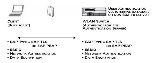
FIGURE 10-32 802.1x Authentication with Termination on WLAN Switch
