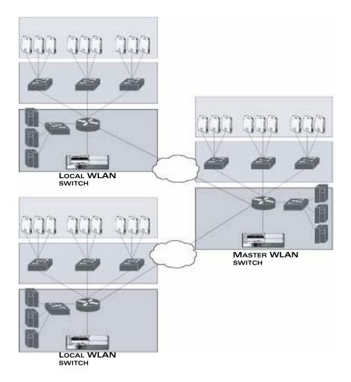
FIGURE 1-4 Master and Local WLAN Switches
